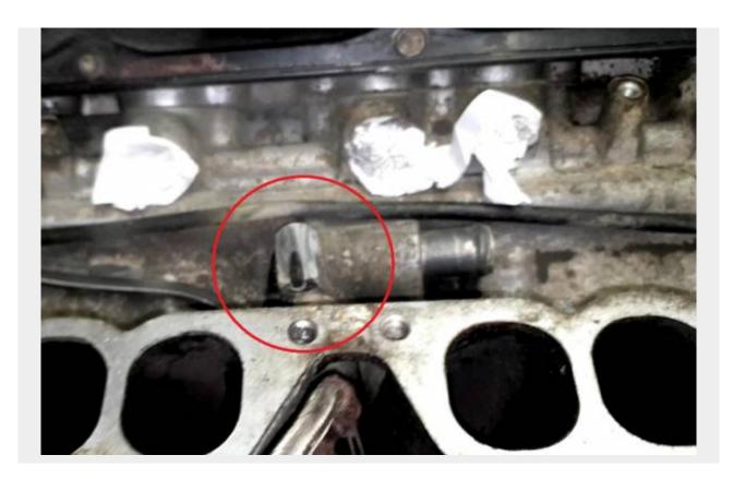
• You can plug the hole from the dispenser by screwing a metal plate with sealant to this place.
